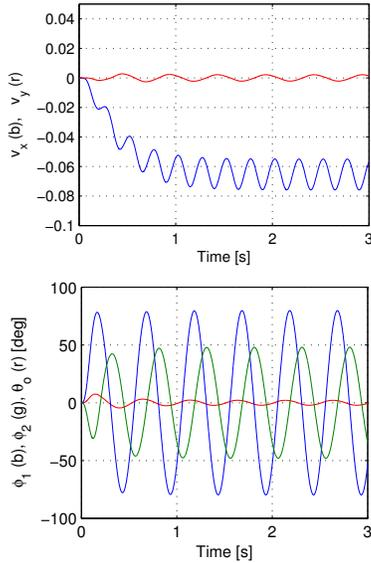
**Figure 2.** Time responses to  $u = 30 \sin(4\pi t) \mu\text{Nm}$
